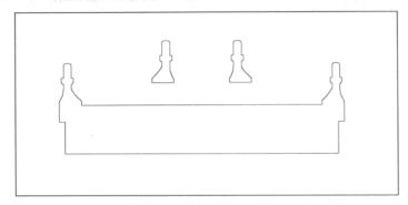
These components can be used with scratchbuilt models, our own components or a replacements for the plastic components supplied with the Ian Kirk kits. Note: the thickness of the Kirk solebars means that they will need to thinned to clear the etched truss posts, and the etched truss posts reduced in width.
